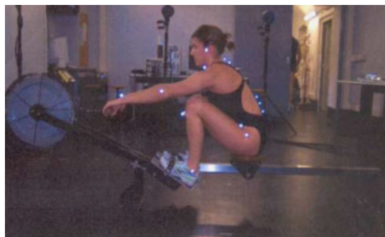
Figure 8. Three-dimensional motion analysis during ergometer rowing: body landmarks are marked with retroreflective markers. In the background, two of the TV cameras can be seen.
